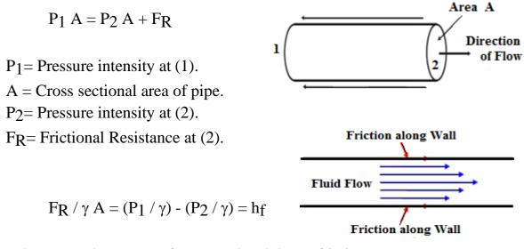
Where, $h_f = Loss$  of pressure head due to friction. $\gamma = Specific$  gravity of water.
