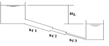
Friction losses through the pipe line are the sum of friction loss of each pipe.
